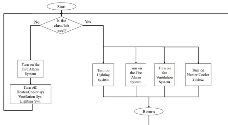
Figure 12: Flow diagram for the working of the second subsystem
