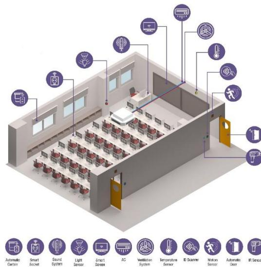
Figure 15: The implementation of the smart system in the laboratory
