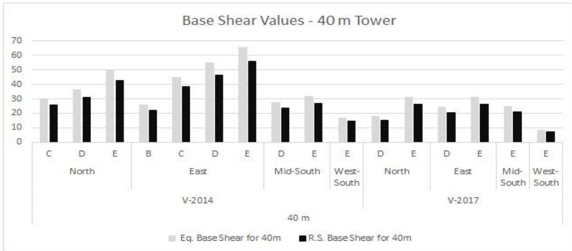
Figure 2: Base shear values – 40 m tower
