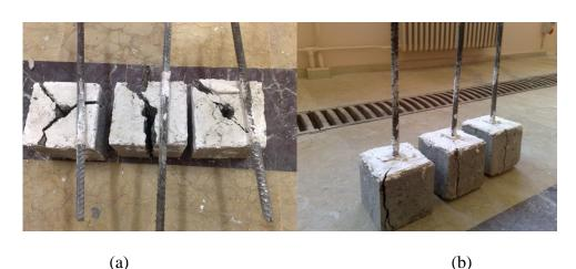
Figure 6: Typical failure patterns of concretes a) without fiber reinforcement and b) with fiber reinforcement
