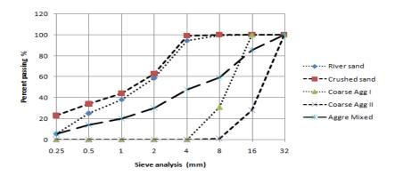
Figure 1: Grading of aggregate
