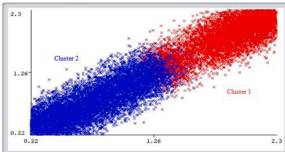
Fig. 13. Cluster formation for pressure during the normal performance (X & Y-axes are in kg/cm<sup>2</sup>).
