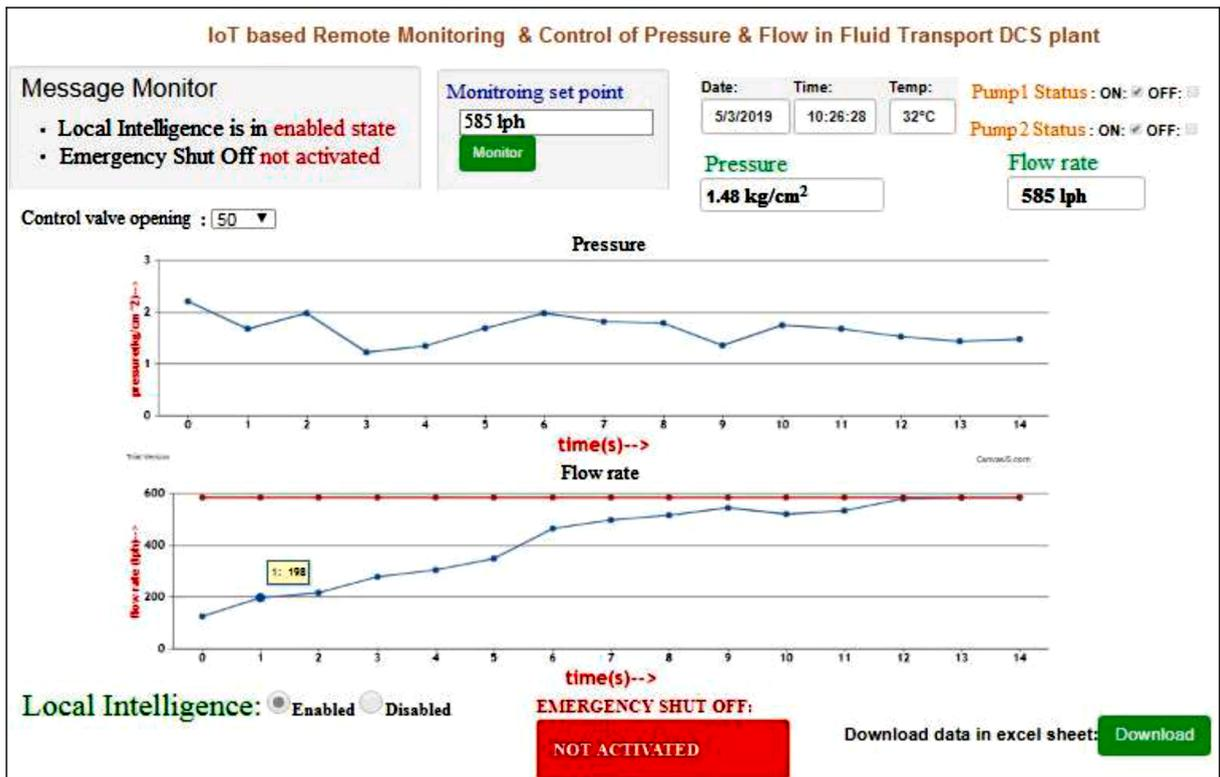
Fig. 11. IoT front end panel to monitor and control pressure and flow rate remotely.
