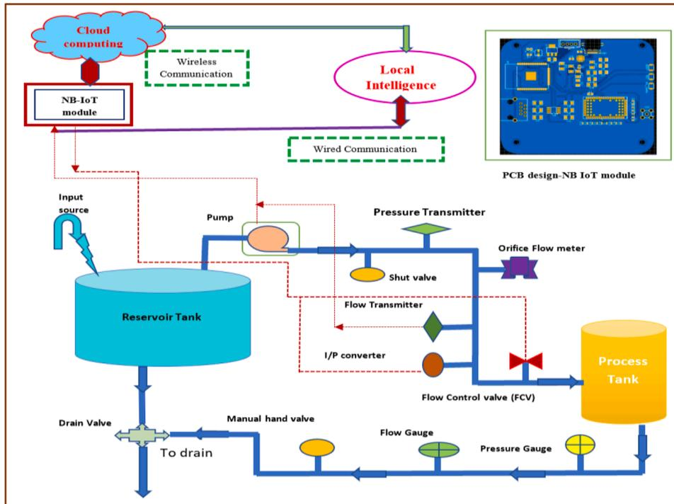
Fig. 5. Interfacing the NB-IoT module with the fluid transportation system.
