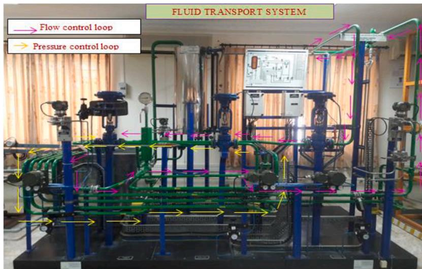
Fig. 2. The lab-scale experimental setup of the fluid transport system.
