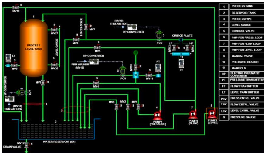
Fig. 3. SCADA view of the lab-scale experimental fluid transport system.
