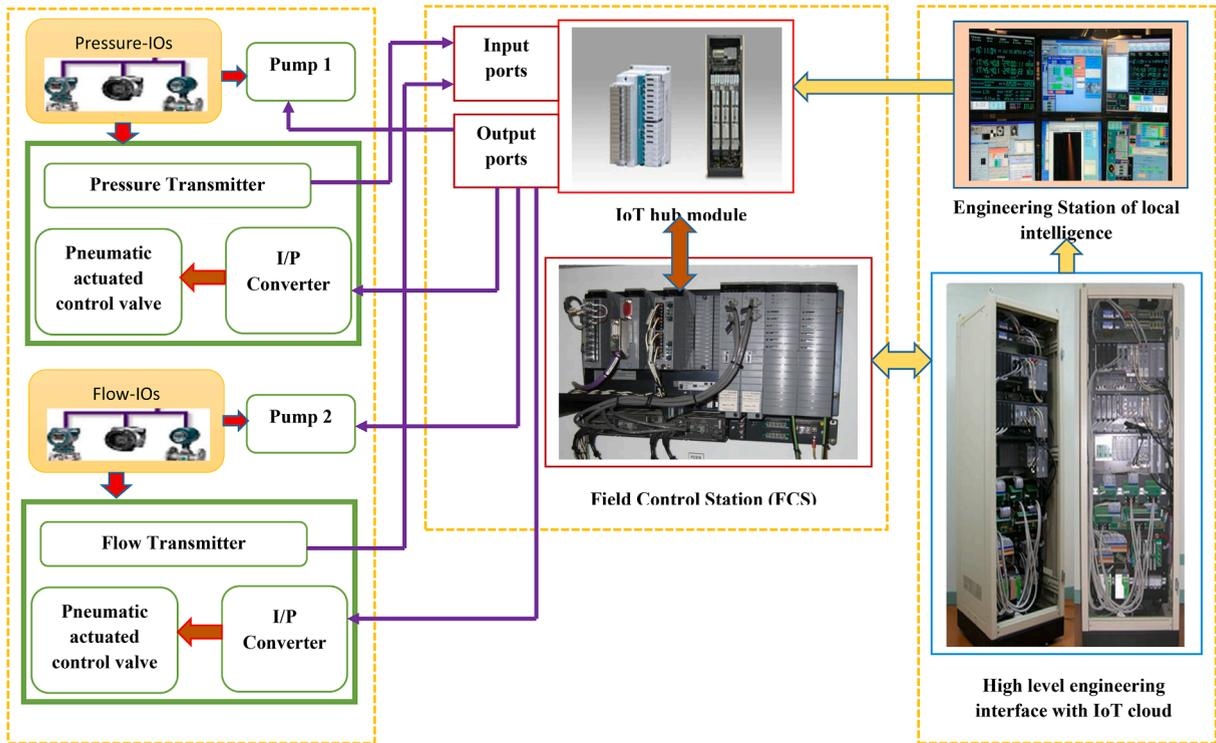
Fig. 1. IoT based architecture with local intelligence for the process.
