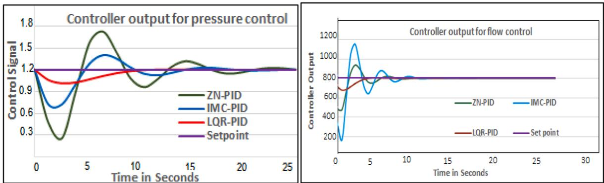
Fig. 9. Controllers output signals for pressure and flow control in the DCS fluid transportation system.
