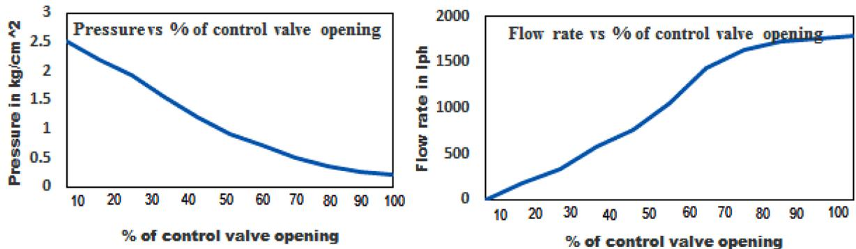
**Fig. 6.** Real-time recorded pressure and flow rates of the fluid for the different level of control valve opening.**Table 3**
