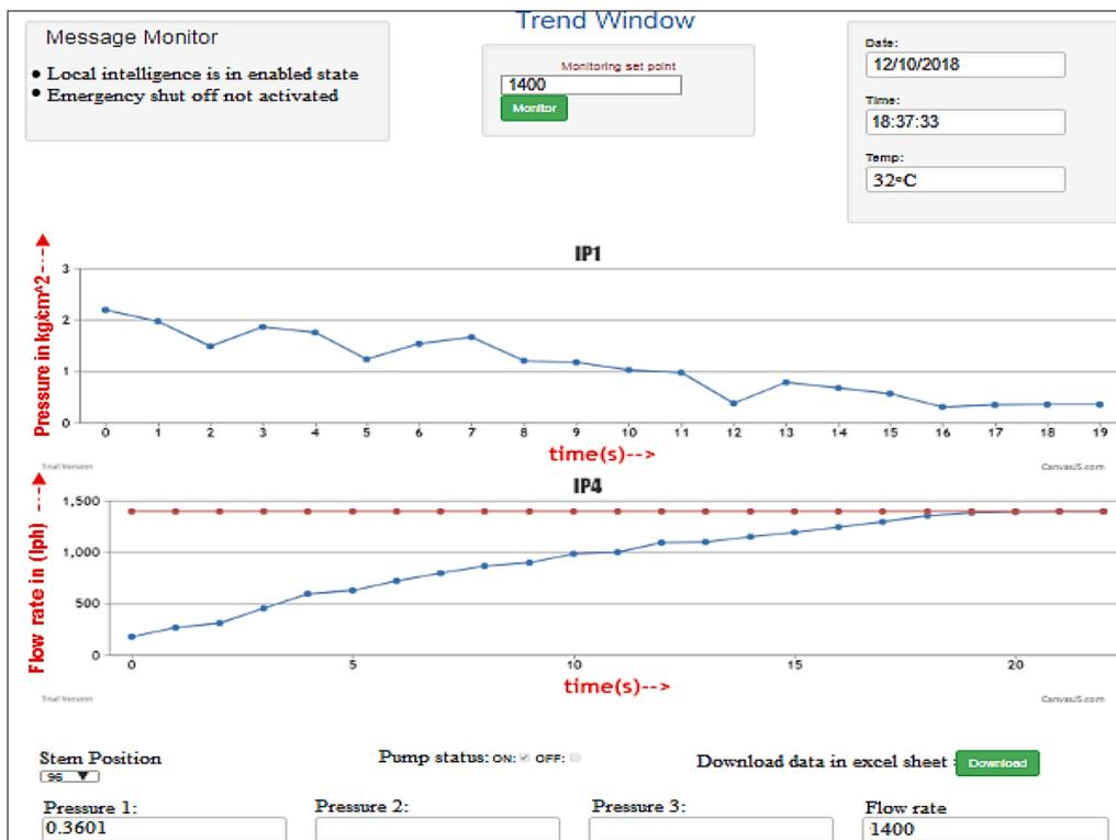
Fig. 7. Real-time monitoring and control of pressure and flow using a Local Intelligence at a field control station.
