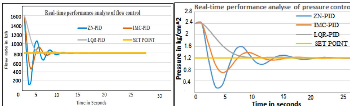
Fig. 8. Real-time performance analyses of pressure and flow rate using ZN, IMC and LQR-PID controller.
