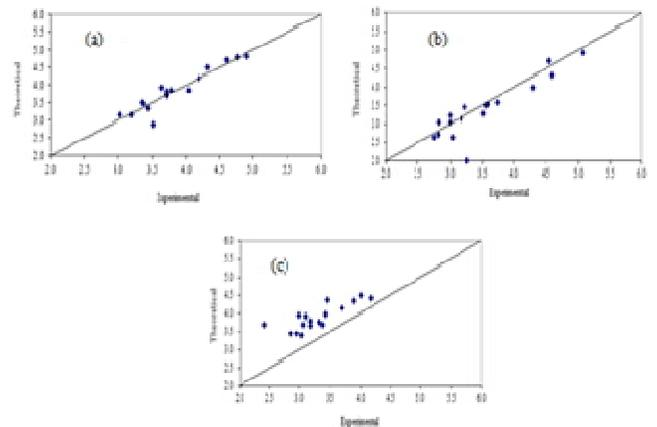
**Figure 4:** Predicted (Theoretical) versus experimental results of ( $f_{sp}$ ) in MPa : a- initial; b- after 1st stage; c- after 2nd stage
