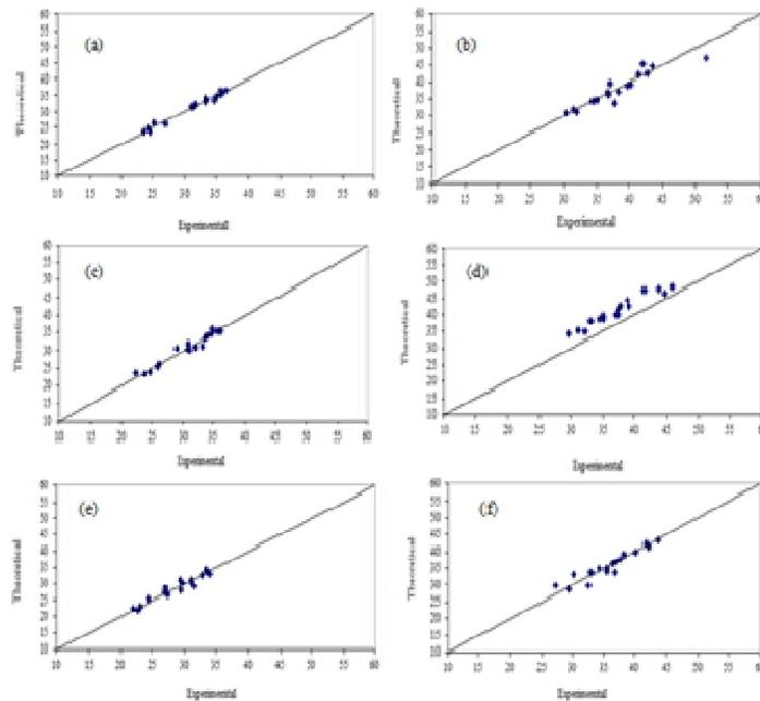
**Figure 2:** Predicted (Theoretical) versus experimental results of ( $f_{cr}^7$ ) in MPa: a-at 7 days; b- at 28 days; c- 7 days (1st stage); d- 28 days (1st stage); e- 7 days (2nd stage); f- 28 days (2nd stage)
