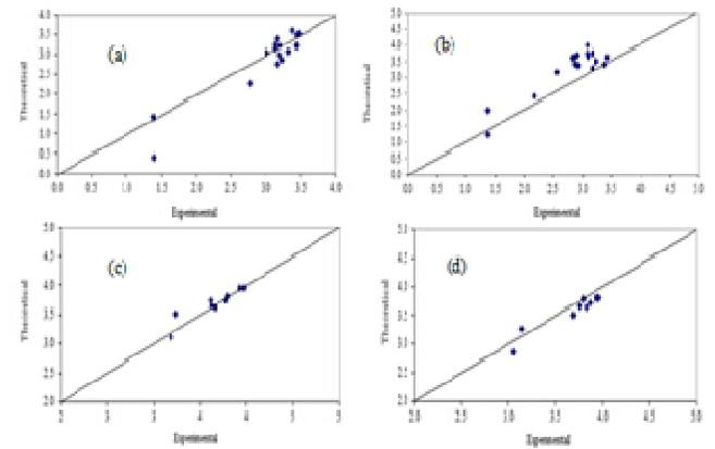
**Figure 5:** Predicted (Theoretical) versus experimental results of modulus of elasticity in(\*10 GPa): a- static ( $E_{cr}^7$ ); b- static after 2nd stage ( $E_{cr2}^{28}$ ); c- dynamic after 1st stage ( $E_{dyn1}^7$ ); d- dynamic after 2nd stage ( $E_{dyn2}^7$ )
