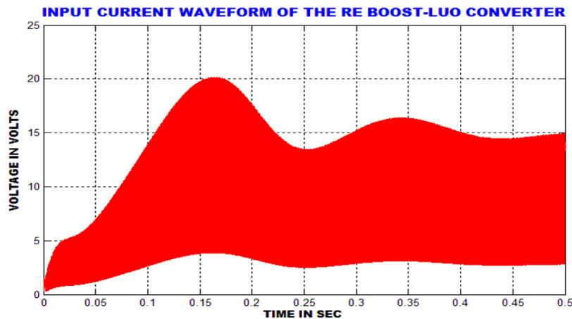
Fig. 8. Simulation result of input current waveform of the DC-DC converter.
