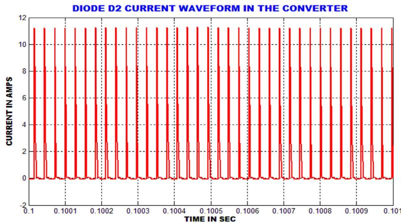
Fig. 11. Current through Diode D2 of proposed converter.
