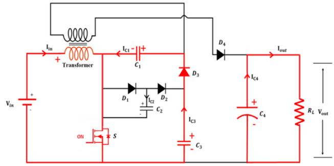
Fig. 2. Switch on mode condition flow diagram.
