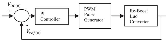
Fig. 6. Closed loop PI controller of the proposed converter.
