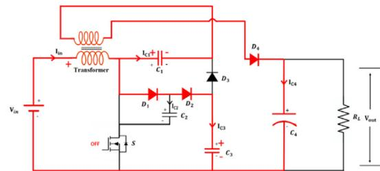
Fig. 3. Switch off mode condition flow diagram.
