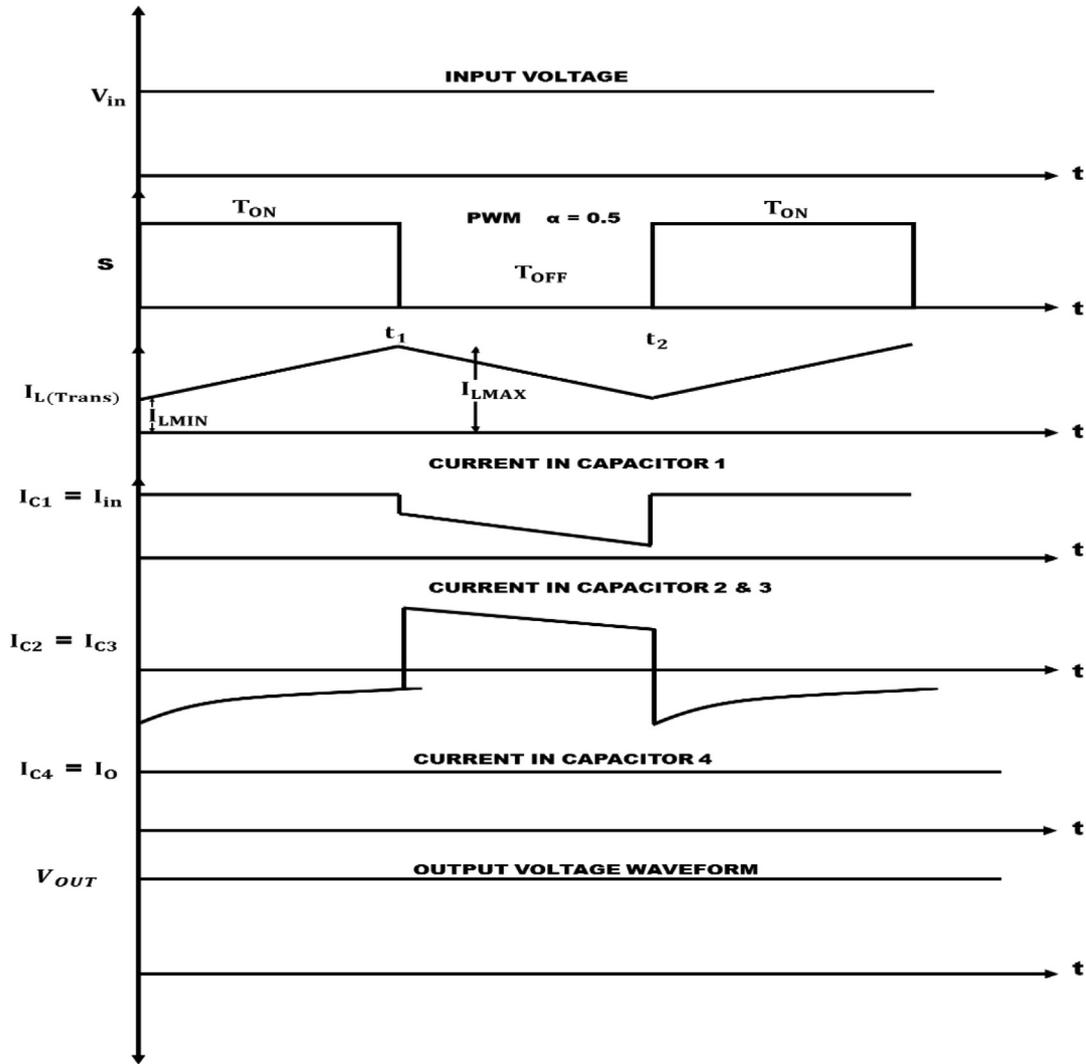
Fig. 4. Switching waveform of proposed Re Boost Luo converter.
