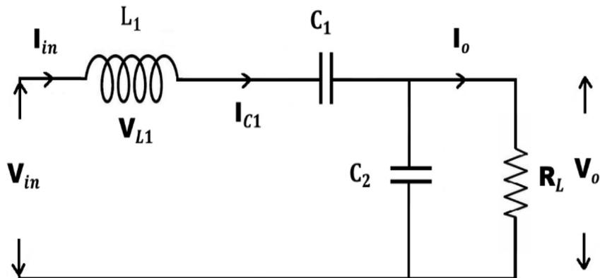
Fig. 5. Elementary circuit of Luo converter.
