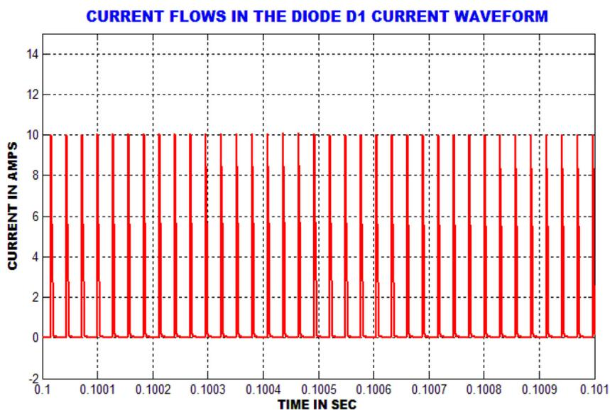
Fig. 10. Current through Diode D1 of proposed converter.
