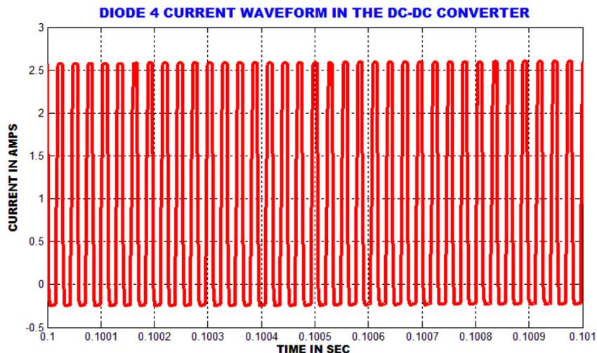
Fig. 13. Current through Diode D4 of proposed converter.
