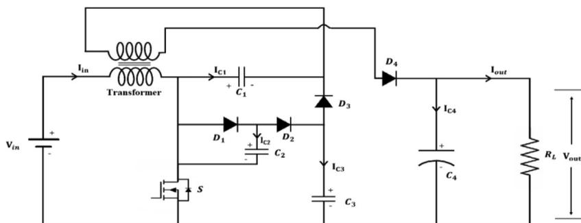
Fig. 1. New topology of DC-DC Re-Boost Luo converter.
