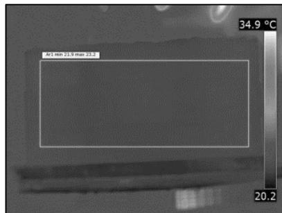
Figure 21: Masonry water tank with average surface temperature of 22.4 °C
