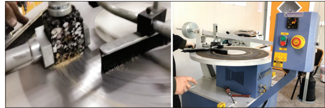
Figure 6: Bohme abrasive wheel abrasion test machine
