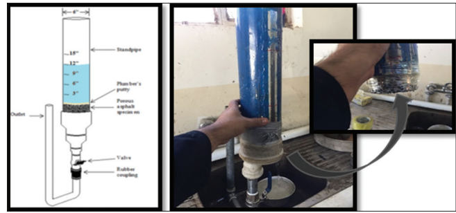
Figure 5: Permeability test schematic
