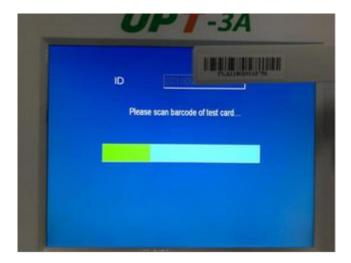
7. Scan the barcode on the back of the test card in the infrared area at the upper right corner of the instrument according to the prompt;
