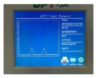
9. The test results can be read out later on the instrument interface. (Press the "Return" or "Continue" in the lower right corner to test the next sample).
