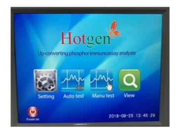
2. Enter into the working interface after pre-heating process. Press "Setting" and then press "read para"
