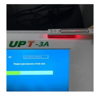
8. After the scan is completed, insert the test card to the bottom according to the prompt;
