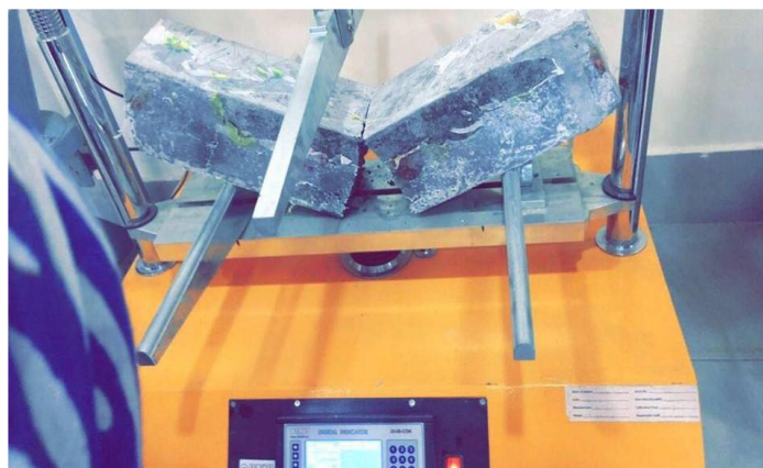
Figure 3: Flexural machine test
