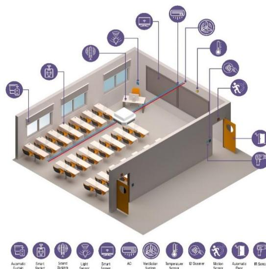
Figure 13: The implementation of the smart system in the class hall
