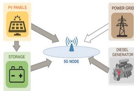
FIGURE 2: Power supply for a 5G site with solar panels and diesel generator in case the power grid is not available.
