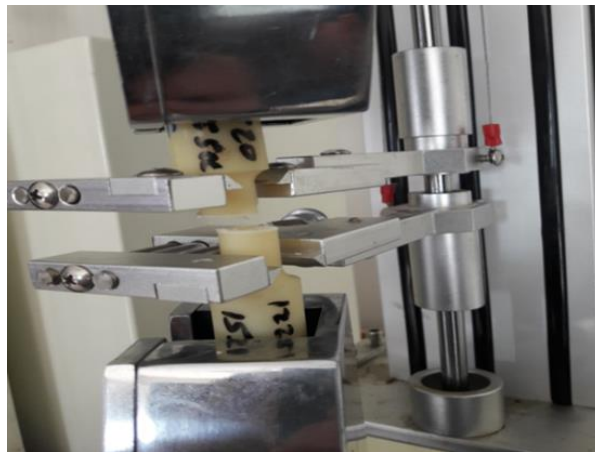
Figure 7: Welded ABS terpolymer of specimen at fracture
