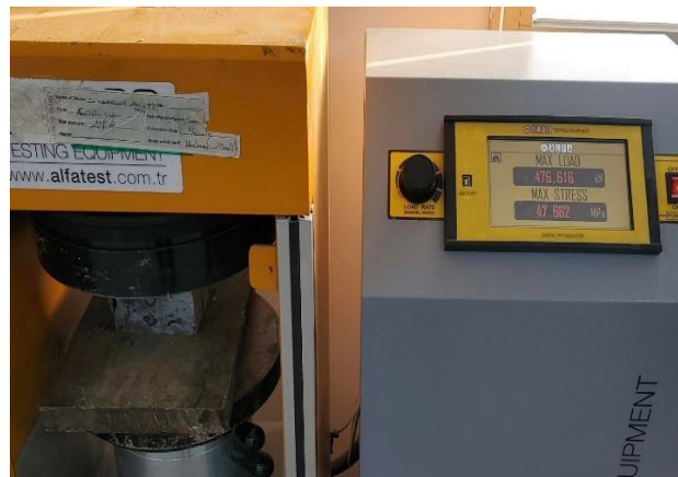
Figure 5: Testing cubes for compression
