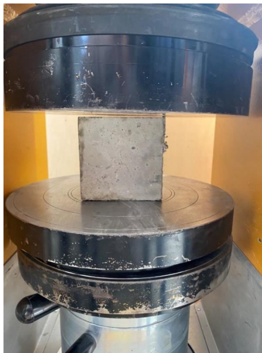
Fig. 7. Specimen under compressive machine test.
