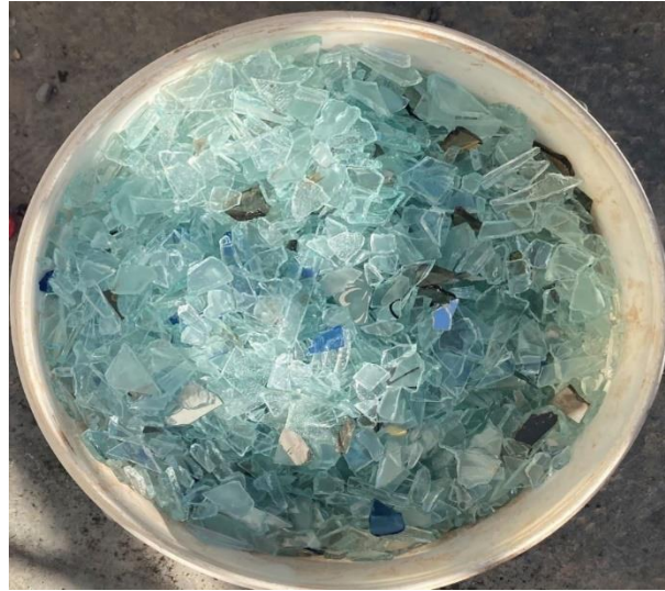
Fig. 2. Crushed glass utilized as a partial replacement for coarse aggregate in concrete.
