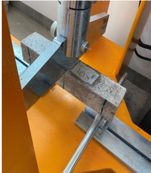
Fig. 9. Prism specimen under the flexural test.
