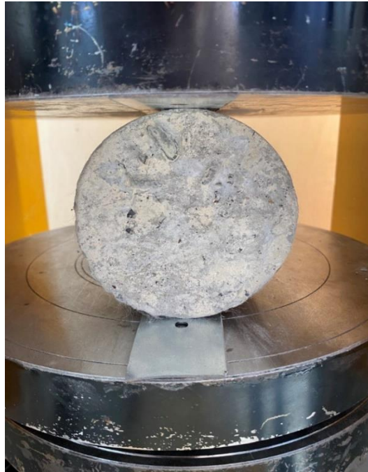
Fig. 8: Splitting tensile test for the cylinder.
