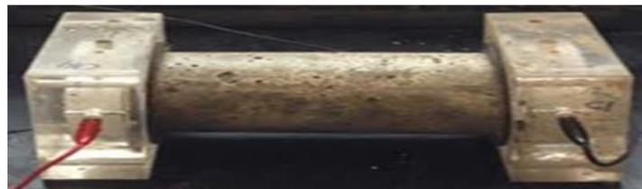
Figure 1: Electrical Resistivity Apparatus
