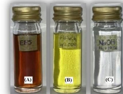
Figure 2: The stock solutions used in the preparation of AuNPs. (A) Lactobacillus CFCS, (B) stock solution of (\text{HAuCl}_4 \cdot x\text{H}_2\text{O}) , and (C) stock solution of (\text{NaOH}) .
