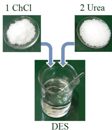
Figure 3: Graphical representation of formation DES from 1 ChCl and 2 Urea
